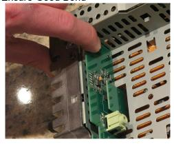
8. Insert Audio Cable into AuxMod Jack and Ensure Plug is Fully Inserted
